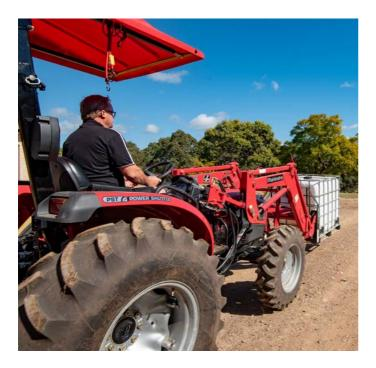
**HEAVY DUTY FRONT AXLE** The heavy-duty front axle ensures maximum reliability in loader and field operations. The bevel gear front axle with a responsive hydrostatic steering provides a tight steering angle, so getting in and out of confine areas is easy.
